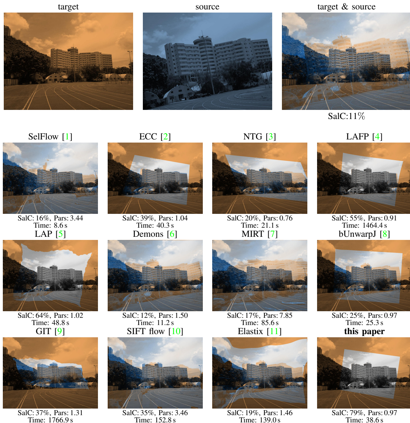
Fig. S4. Registration of real images (960 × 1280 pixels) that have undergone large rotation and scaling, using different algorithms (expanded from Fig. 8).
